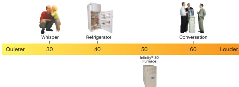
Carrier manufactures gas furnaces that are among the quietest in the industry. We test our products in a sound laboratory specifically built to resemble a typical residence. Sound level recordings produced at steady state, low fire operation (the most common operating condition), measured 3 feet from furnace. Other sound levels, mentioned for comparison, as published at <http://www.nidcd.nih.gov/health/hearing/ruler.asp>.
