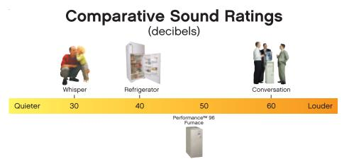
Carrier manufactures gas furnaces that are among the quietest in the industry. We test our products in a sound laboratory specifically built to resemble a typical residence. Sound level recordings produced at steady state, low fire operation (the most common operating condition), measured 3 feet from furnace. Other sound levels, mentioned for comparison, as published at http://www.nidcd.nih.gow/health/hearing.ruler.asp.
